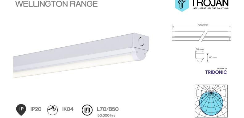
The Wellington LED batten luminaire has been meticulously crafted to meet the highest standards of specifications and energy-saving requirements. It features Tridonic LED boards and driver, polycarbonate diffuser and an aluminium housing tcomplete with standard BESA and conduit mounting points on the rear.
