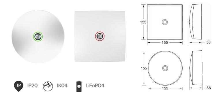
The Marland Range is a surface mount standalone emergency LED luminaire which incorporates either pen area or corridor LEDs. The unit is designed for non-maintained use. This product operates with the latest LiFePO4 batteries that offer a long life and a low parasitic load.
