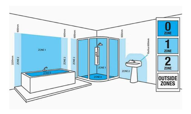
Zone O is inside the bath or shower itself. Any fitting used in this zone must be low voltage, (max 12v) and be rated at least IP67 which is total immersion proof.
